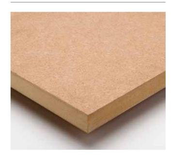
Medium Density Fibreboard (MDF) is engineered board produced from resin bonded wood fibers under high pressure and heat.
