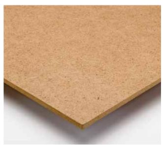
HDF is an engineered board produced from resin bonded wood fibers under high pressure and heat. HDF is a non-load-bearing product for interior use in dry conditions. HDF, due to its very fine surface, is suitable for different coatings – veneering, laminating, painting and varnishing. Kronospan HDF is available in a variety of thicknesses, and a sanded surface to one or both sides.
