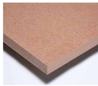
MDF FR are non-load-bearing boards with improved fire retardant properties and are manufactured in compliance with European standard EN 622-5 where they are defined as boards for general use in dry conditions. MDF FR is increasingly used particularly in public spaces where stringent fire regulations must be met. According to EN 13501-1 boards are classified B-s2, d0 in terms of reaction to fire.
